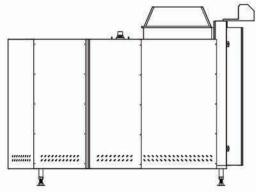
Portable Rotary Oven with fully indirect heat System is designed and provided for baking Lavash, Taftoon, Barbary, Sheermal Breads and as well as Pizza with traditional appearance and good taste by utilizing of punched (Lavash Bread), flat (Barbary & Taftoon Breads) and bumpy (Sangak Bread) cast iron baking plates.
